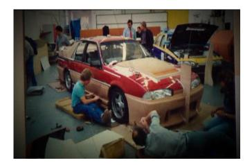
The "Walkinshaw" was designed to achieve a level of aerodynamic efficiency that was lacking in road cars of the time. The body kit had 27 individual fiberglass components. The high boot spoiler was found in the wind tunnel to be the only way to prevent the VL's rear lifting at speed. It proved itself when it won Bathurst in 1990, under "Group A" regulations.
