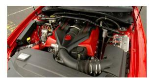
In HSV form it delivered 297kW at 6,000 rpm. The engine had great flexibility with 87% of peak torque available from as low as 1,600 rpm.
