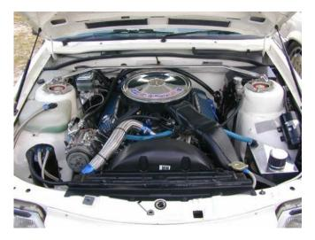
Thus, in conjunction with Holden's engineers, the 308 was revised, a 1 mm shorter stroke giving it a capacity of 4987 cc. Instead of the expensive Carillo connecting rods used on the Group C cars, L 34 rods were fitted. Surprisingly, instead of resulting in a loss of performance, power output actually rose from 177 kW at 4500 rpm to 196 kW at 5200 rpm.
